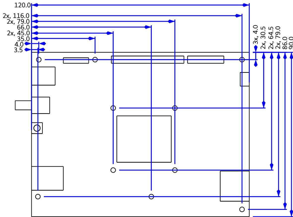
View 1: Mounting holes and overall size (top view)
