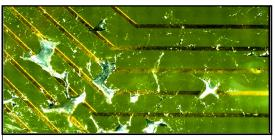
UNACCEPTABLE SOLDER SPLATTER
