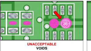
Bubbles and voids in the adhesive reduce the deposit's cross-section and retention properties. NASA-STD-8739.2 [ 8.9 ], [ 8.10.1 ]
