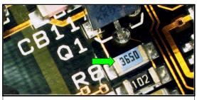
PREFERRED Part markings are visible and oriented uniformly. NASA-STD-8739.2 [ 8.7.4.a ], [ 12.7.1.b ], [ 12.8.1.f ]
