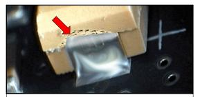
UNACCEPTABLE DAMAGED PART SEAL Parts with damaged seals shall not be used. NASA-STD-8739.2 [ 12.7.2.b ]
