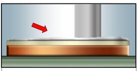
UNACCEPTABLE INSUFFICIENT SOLDER QUANTITY The solder quantity shall be sufficient to form a properly wetted, concave fillet.
