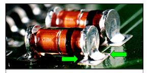
**PREFERRED** The termination exhibits a concave fillet on the terminal faces, with evidence of good wetting to the metallization and the periphery of the land.
