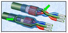
ACCEPTABLE SHIELD TERMINATION – CRIMP SLEEVE
