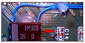
UNACCEPTABLE IMPROPER MOUNTING ORIENTATION
