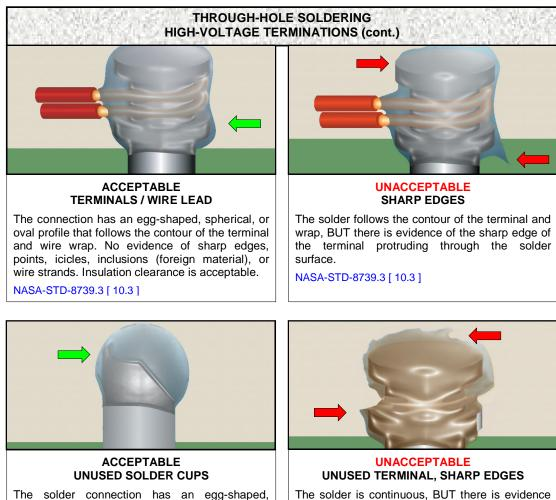
spherical, or oval profile. No evidence of sharp
