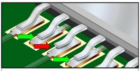
UNACCEPTABLE IMPROPER COPLANARITY
