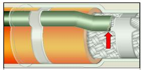
UNACCEPTABLE INSUFFICIENT INSULATION CLEARANCE
