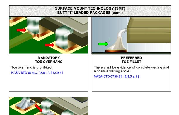
UNACCEPTABLE MISSING TOE FILLET There shall be evidence of complete wetting and a positive wetting angle that extends over the complete periphery of the connection.
