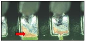
UNACCEPTABLE IMPROPER TINNING
