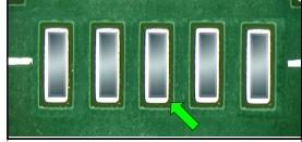
ACCEPTABLE SOLDER PREFORM APPLICATION The preforms are applied with proper alignment and placement.
