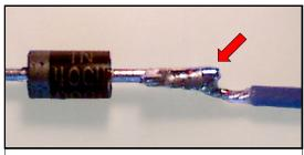
UNACCEPTABLE LEAD / CONDUCTOR MISALIGNMENT
