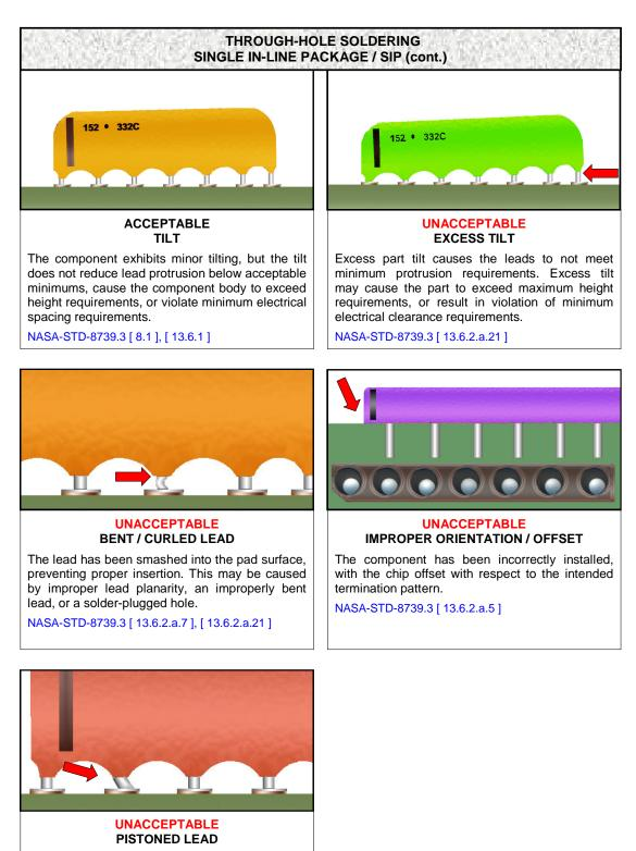
The lead has been displaced vertically (pistoned) during insertion. This may be caused by improper lead planarity, an improperly bent lead, or a solder-plugged hole.
