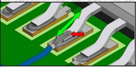
UNACCEPTABLE IMPROPER LAP TERMINATION GULL WING SMT
