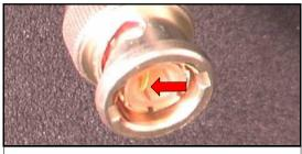
**UNACCEPTABLE IMPROPER ASSEMBLY CENTER CONTACT(S)**
