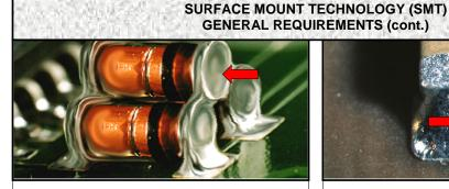
UNACCEPTABLE PIGGYBACKED PARTS Piggybacking, or stacking, of parts not designed specifically for that configuration is prohibited. NASA-STD-8739.2 [ 8.7.4.e ], [ 12.6.2.a.1 ]
