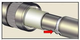
**UNACCEPTABLE EXCESS / IMPROPER SOLDER**
