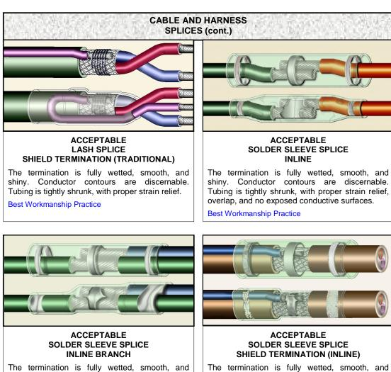
The termination is fully wetted, smooth, and shiny. Conductor contours are discernable. Tubing is tightly shrunk, with proper strain relief, overlap, and no exposed conductive surfaces.
