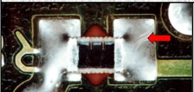
UNACCEPTABLE SCRATCHES (SOLDER FILLET) Scratches in the solder are prohibited. NASA-STD-8739.2 [ 12.8.2.b.14 ]
