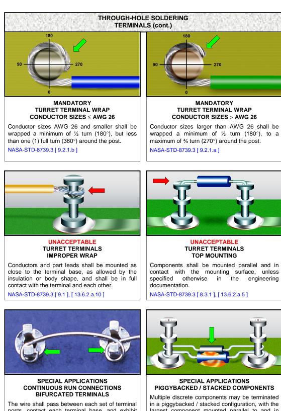
posts, contact each terminal base, and exhibit stress relief. The wire ends shall be attached to the first and last terminal with a 90° to 180° wrap. NASA-STD-8739.3 [ 9.3.4 ]
