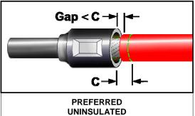
The contact has been deformed only by tool indenters. Indents are symmetrical and centered on the crimp barrel. No exposed base metal or other damage. Proper insulation spacing (C). NASA-STD-8739.4 [19.6.1.c]
