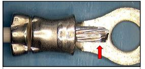
UNACCEPTABLE EXCESSIVE CONDUCTOR LENGTH
