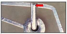
UNACCEPTABLE IMPROPER LEAD LENGTH
