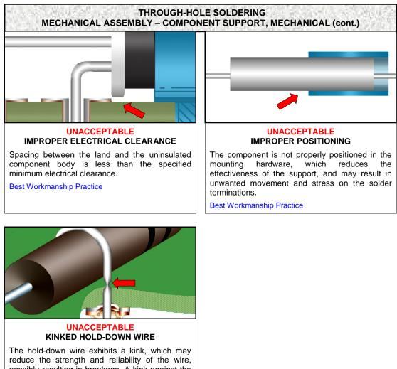
The hold-down wire exhibits a kink, which may reduce the strength and reliability of the wire, possibly resulting in breakage. A kink against the component body may result in component damage or failure.
