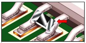
UNACCEPTABLE IMPROPER MOUNTING SMT COMPONENTS MOUNTED ON LEADS
