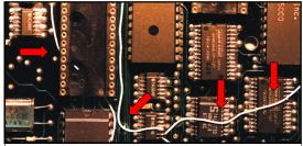
UNACCEPTABLE IMPROPER ROUTING (OVER / UNDER COMPONENTS)
