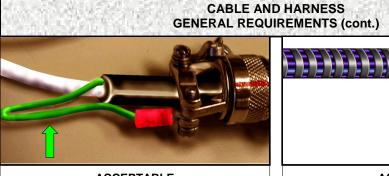
ACCEPTABLE SHIELD / DRAIN WIRE
