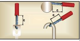
UNACCEPTABLE IMPROPER INSULATION GAP (C)
