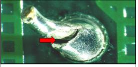
UNACCEPTABLE FRACTURED SOLDER
