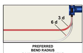
**COAXIAL RIBBON CABLE** The bend radius for coaxial ribbon cables shall not be less than six (6) insulated wire diameters short-term, ten (10) diameters long-term.
