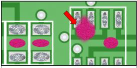
UNACCEPTABLE ADHESIVE ON LEADS / SOLDER PADS
