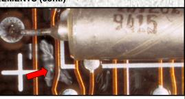
UNACCEPTABLE FLUX SPLATTER
