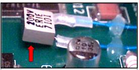
UNACCEPTABLE IMPROPER STAKING
