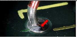
UNACCEPTABLE SCRATCHES (SOLDER FILLET) Scratches in the solder are prohibited. NASA-STD-8739.3 [ 13.6.2.b.3 ]
