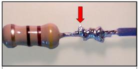
UNACCEPTABLE IMPROPER LASH / WRAP
