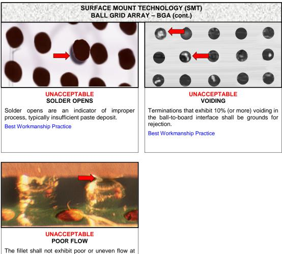
The fillet shall not exhibit poor or uneven flow the top of the solder fillet. Best Workmanship Practice
