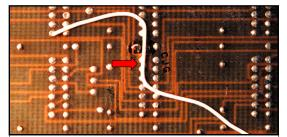
UNACCEPTABLE IMPROPER ROUTING (OVER TEST POINTS)
