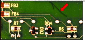
UNACCEPTABLE CRACKS (LAMINATE)
