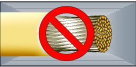
UNACCEPTABLE INAPPROPRIATE CONDUCTOR TYPES Chemical stripping of other than solid, single-
