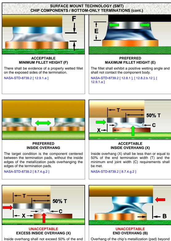
Inside overhang shall not exceed 50% of the end termination width (t) and the minimum end joint width (C) requirements shall be met.
