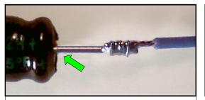
ACCEPTABLE LEAD SEAL / WELD BEAD SPACING The component end of the solder joint shall not be closer than 2 lead diameters or 0.50 mm (0.020 in ) which over in larger from the lead cool
