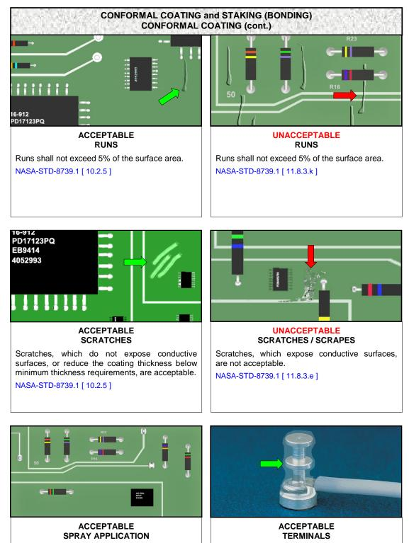
The conformal coating is evenly applied, exhibits uniform color, thickness, proper adhesion, and is smooth and tack free. No evidence of shadowing, orange peel, or dusting.
