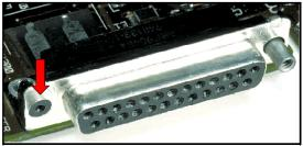
UNACCEPTABLE MISSING MOUNTING / CONNECTING HARDWARE
