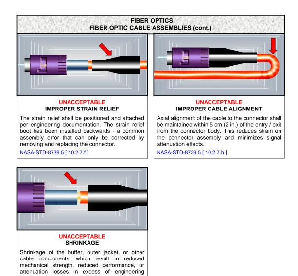
specification, shall be cause for rejection. NASA-STD-8739.5 [ 10.3.3.d ], [ 11.5.3.d ]
