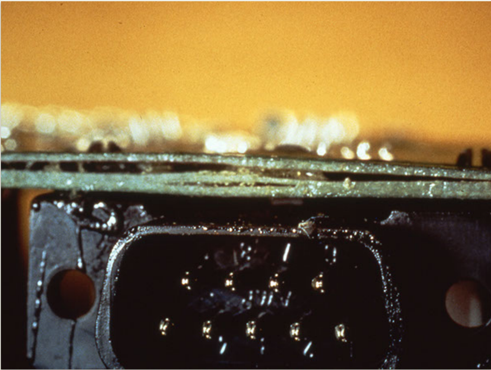
Delamination, base material - Reject
