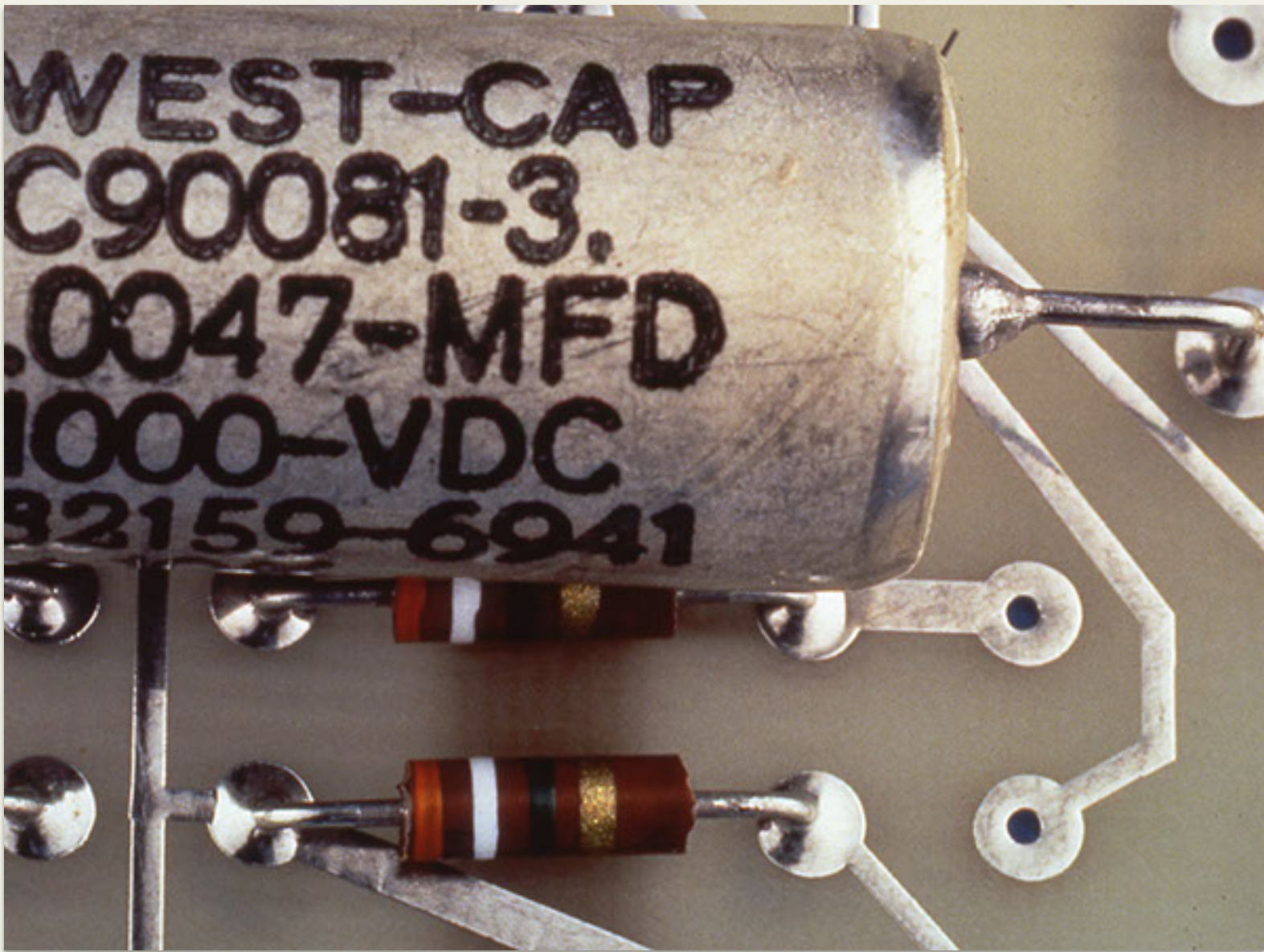
Large component obscures termination of another Part - Reject
