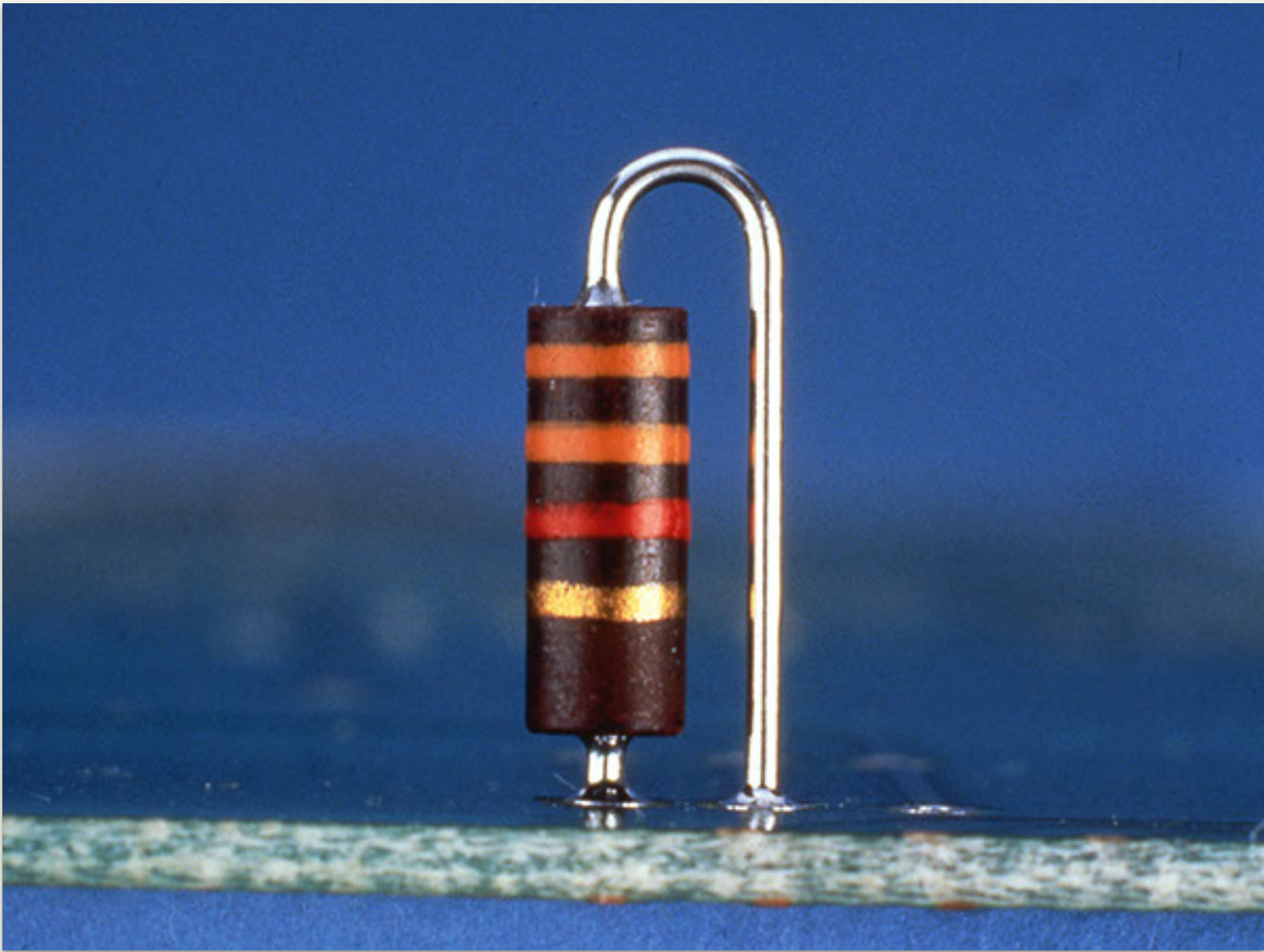
Vertical mounted axial lead component - Accept
