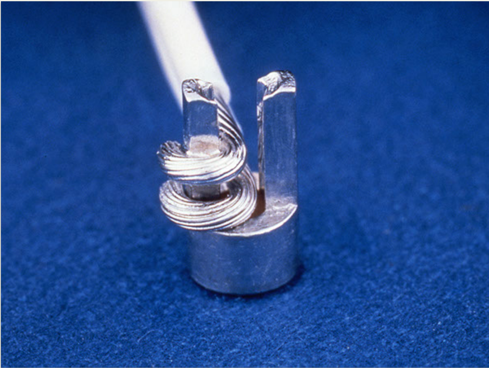
Improper mechanical wrap - Reject
