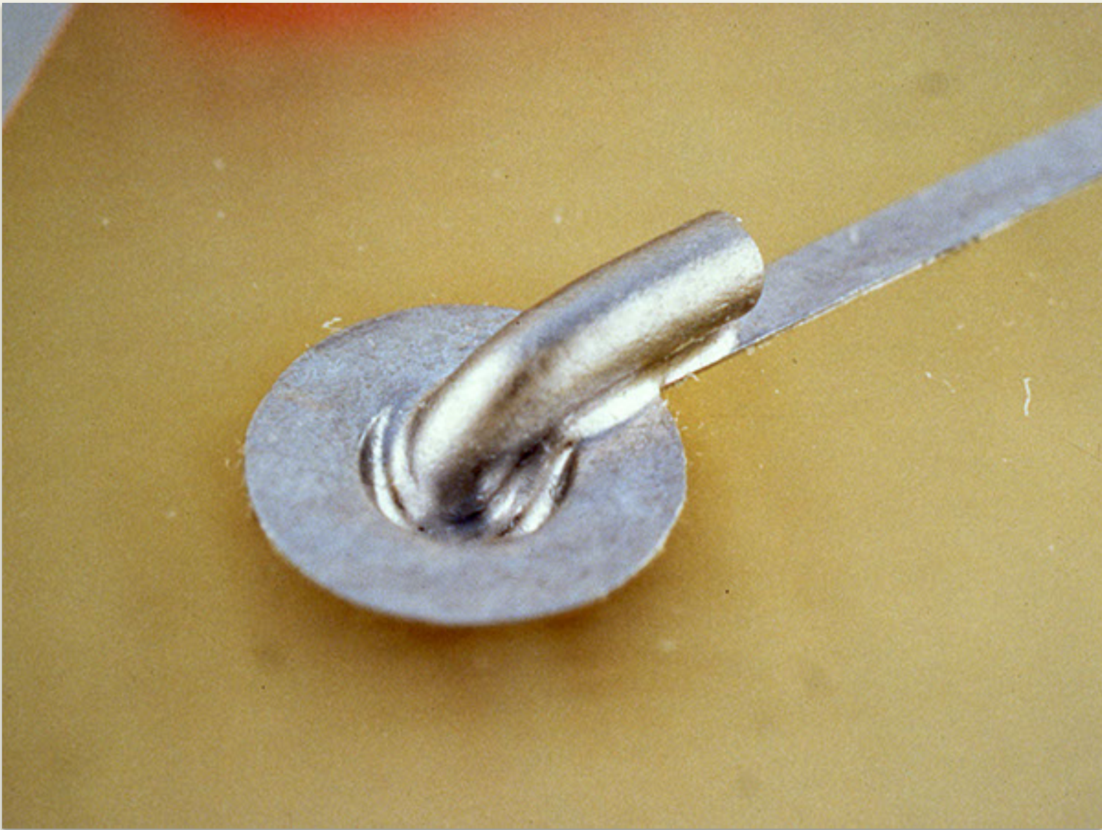
Insufficient solder - Reject
