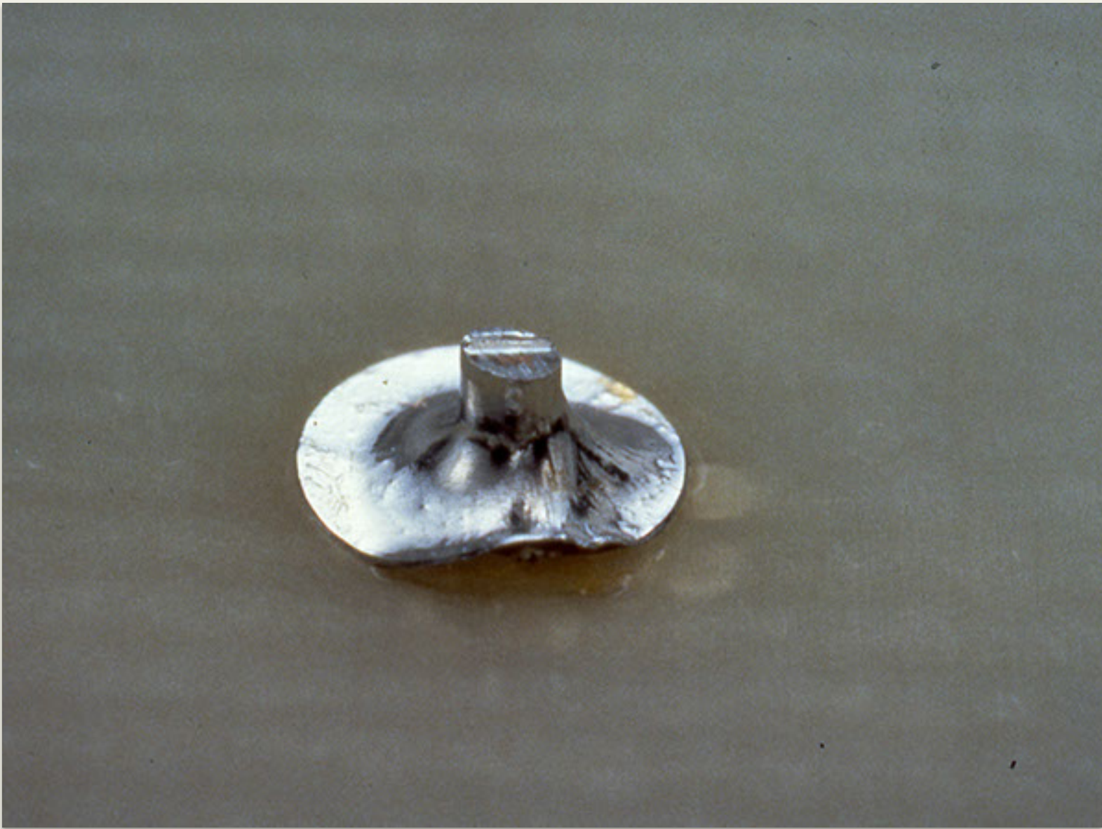
Lifted pad - Reject
