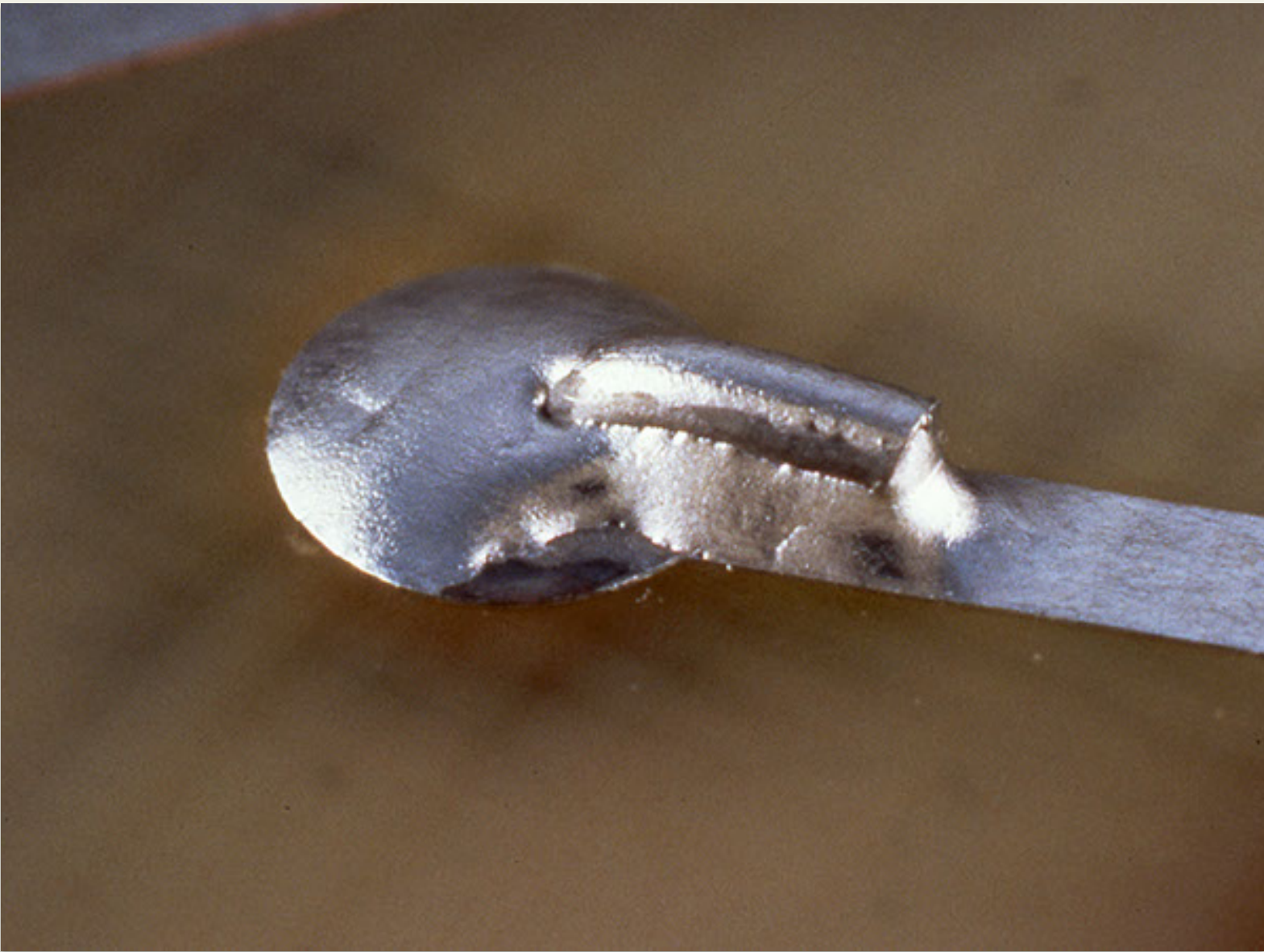
Cold solder, non wetting - Reject
