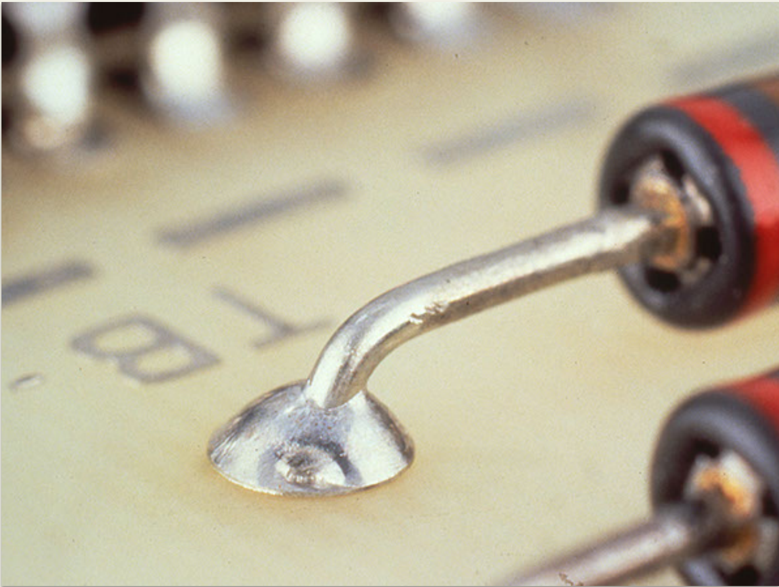
Poor wetting/reflow stress lines - Reject
