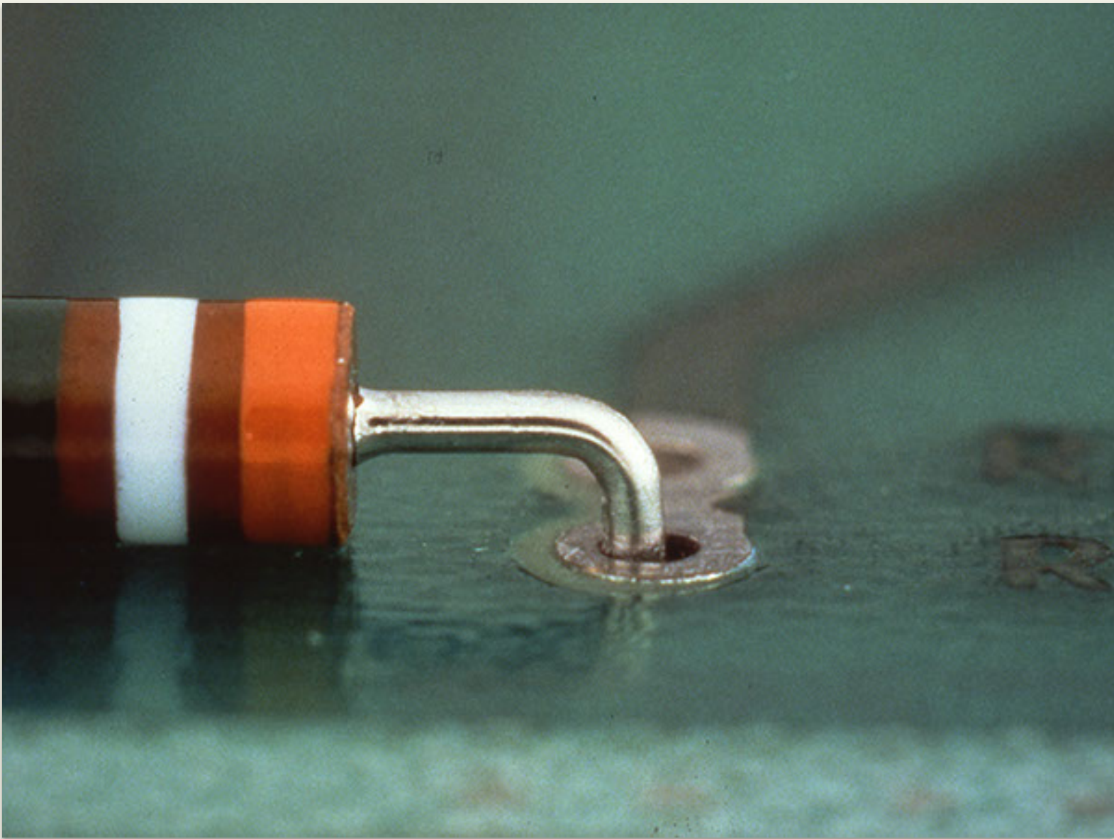
Correct lead bend radius - Accept
