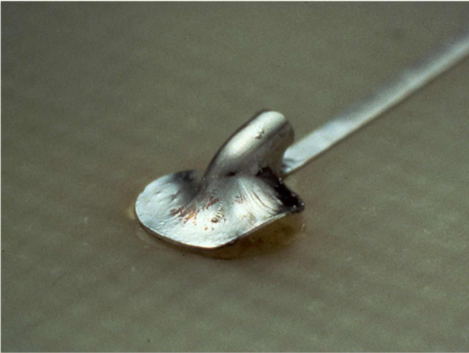
Lifted pad - Reject
