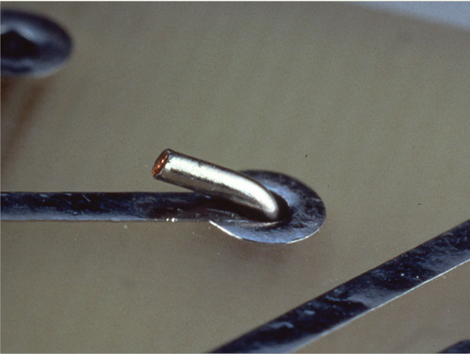
Excessive lead spring back - Reject
