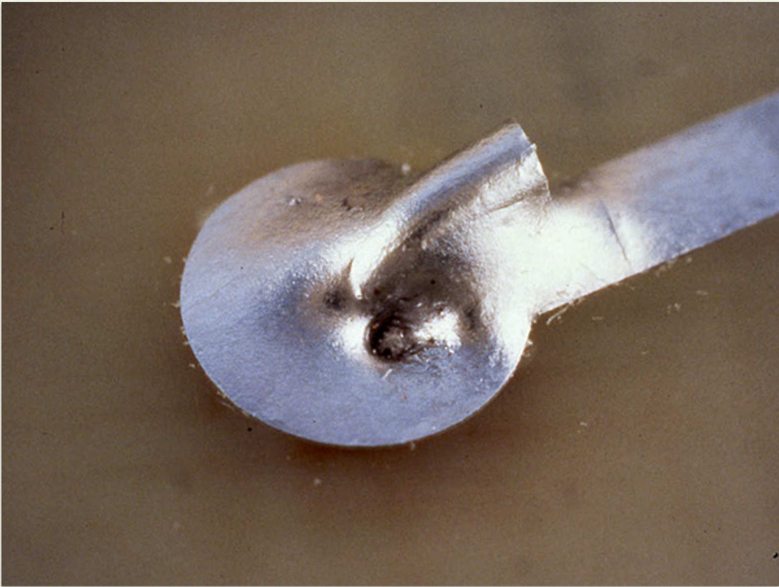
Pit, void - Reject
