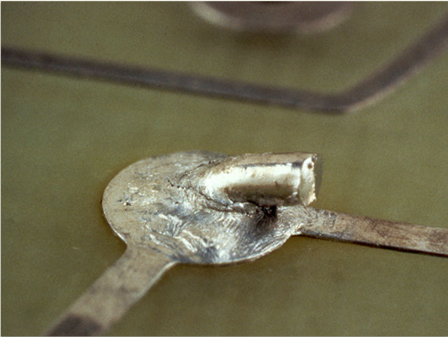
Disturbed solder - Reject
