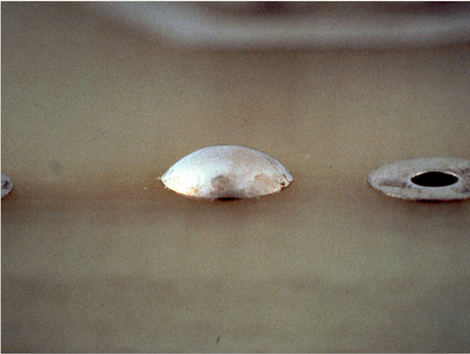
Excessive solder - Reject
