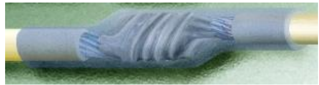
Figure 19-12. Sleeved Lash Splice
