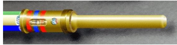
Figure 19-23. Wires Crimped Within Contact
